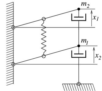
$$\begin{aligned} m_1 x_1'' &= d(x_2 - x_1) + k_2(x_2' - x_1') - k_1 x_1' \\ m_2 x_2'' &= d(x_1 - x_2) + k_2(x_1' - x_2'). \end{aligned}$$
