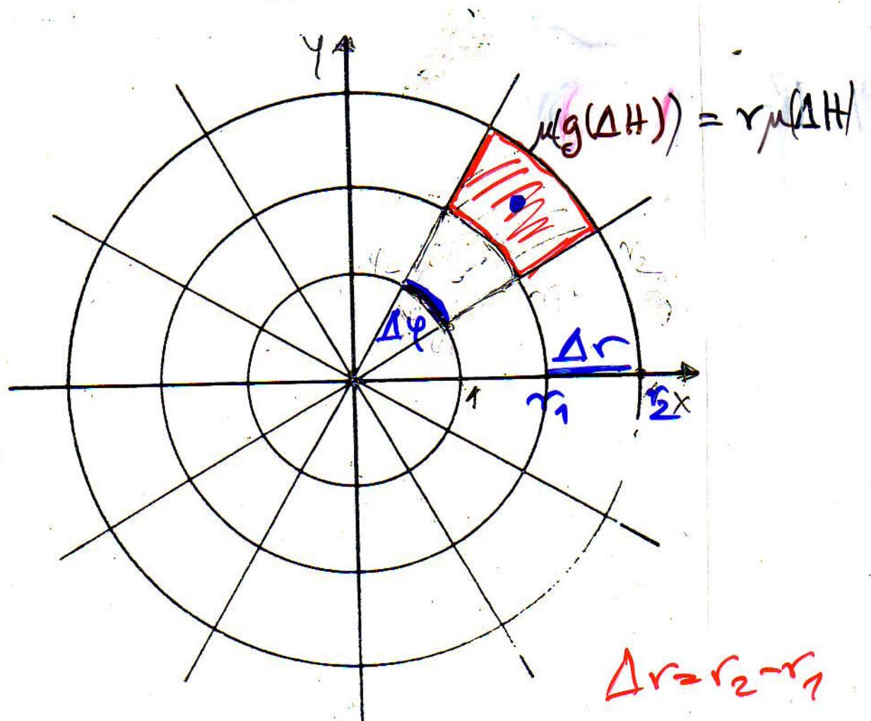
$$\begin{aligned} u(g(\Delta H)) &= \frac{1}{2} \Delta\varphi r_2^2 - \frac{1}{2} \Delta\varphi r_1^2 \\ &= r \Delta\varphi \Delta r \quad r = \frac{1}{2}(r_1 + r_2) \end{aligned}$$
