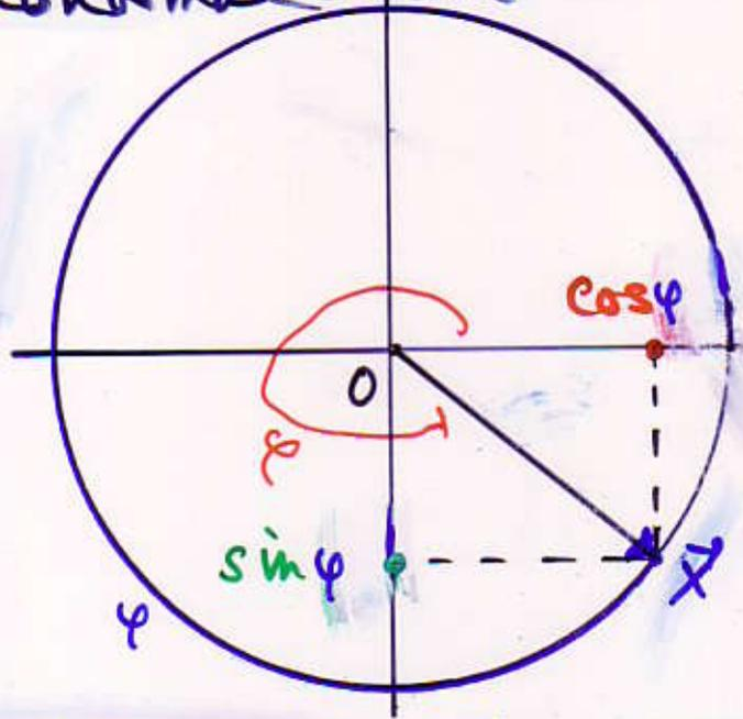
$$\cos \varphi = \langle \vec{e}_1 | \vec{x} \rangle, \quad \sin \varphi = \langle \vec{e}_2 | \vec{x} \rangle$$
